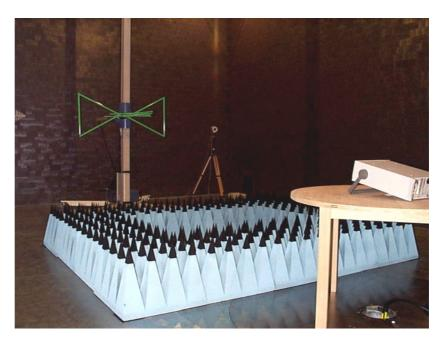
For emission tests, the floor is reflective. For immunity tests, the reflective floor is covered by movable absorber panels (ferrites and pyramidal)
