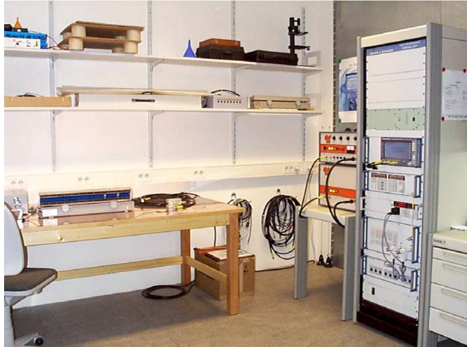
For measurements of RFI Power or shielding effectiveness, an **absorbing clamp MDS21** is placed on the **automatic clamp rail HCA**, controlled by a **HCC**.
